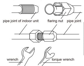
Torque for tightening nut
