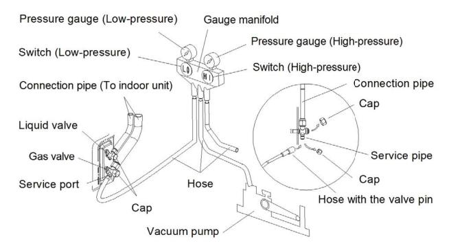
**NOTICE** For large-size units, there are maintenance ports for liquid valve and gas valve. During evacuation, you may connect the two hoses of the branch valve assembly to the maintenance ports to speed up the evacuation.
