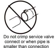
Installation method: Connect the connection pipes first to the unit. When bending a connection pipe, be careful not to damage the pipe. Do not over-tighten the screw nut, otherwise leakage will occur. Besides, the outside of connection pipe should be added with a layer of insulating cotton to protect it from mechanical damage during installation, maintenance and transportation.
