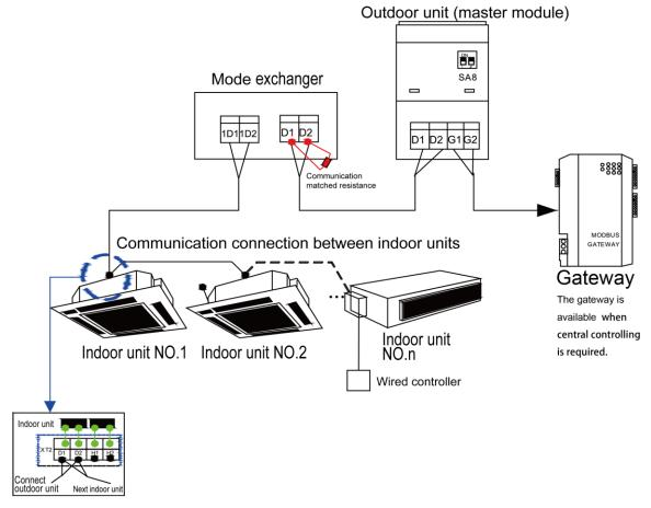
Fig.41 Connection of communication for single-module system and single-module converter system
