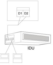
Fig.44 One wired controller controls one IDU
