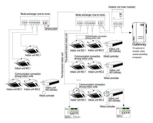
Fig.42 Connection of communication for single-module system and multi-module converter system
