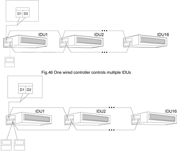
Fig.47 Two wired controllers control multiple IDUs
