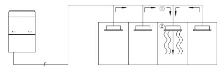
① Flow direction of refrigerant leakage.
