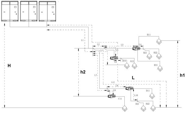
Remark: Equivalent length of one Y-type manifold is about 0.5m (1-3/4ft.).
