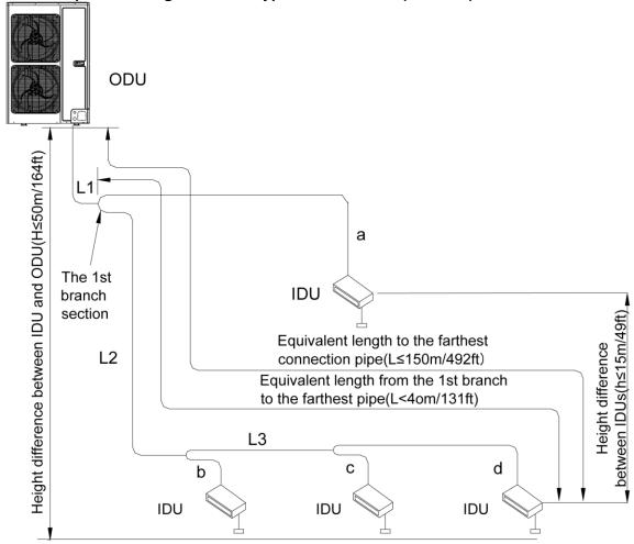
Each Y-type branch equals to 0.5m(1-5/8ft) and each branch header equals to 1.0m(3-1/4ft). Fig.5 Allowable Length and Height Difference of Connection Pipe
