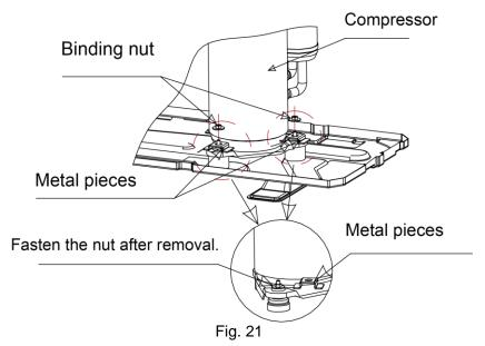
When installing the unit, metal pieces for transportation must be removed. (except for GMV-60WL/A-T(U)) .Then fasten the binding nuts again and wrap back soundproofing cotton.If unit runs with metal pieces fitting on, compressor will shake abnormally and unit's operating life will be shortened.
