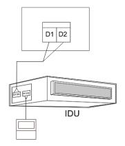
One wired controller controls one IDU
