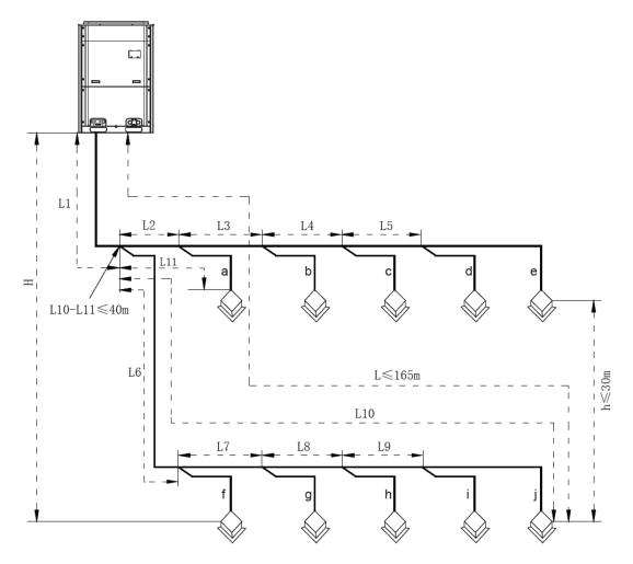
L10: Length from the first branch to the farthest IDU; L11: Length from the first branch to the nearest IDU; Equivalent length of branch of IDU is 0.5m (1-3/4feet).
