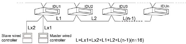
Notes: If the air conditioning units are installed at a place with strong electromagnetic interference, a shielded cable must be used as the communication cable between the indoor unit and wired controller, and a shielded twisted pair must be used as the communication cable between the indoor unit and indoor (outdoor) unit.
