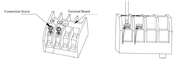
(3) If a single communication wire is not long enough and needs to be connected, the connected joint must be welded or pressure-welded. Do not simply twist the wires together.
