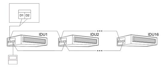
One wired controller controls multiple IDUs
