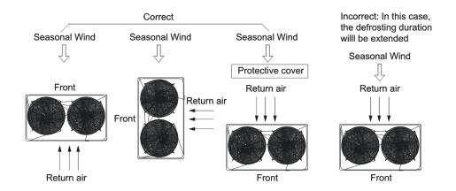
4) Anti-monsoon installation requirements for unit connecting exhaust duct:
