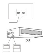
Two wired controller controls one
