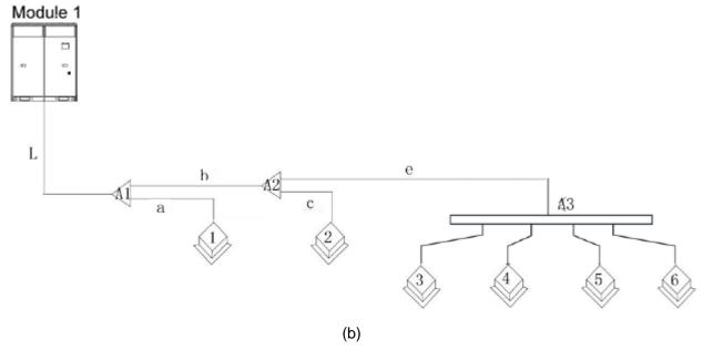
7.3.2 Select appropriate pipe between outdoor unit and the first indoor branch ("L") as per the pipe size of outdoor unit.
